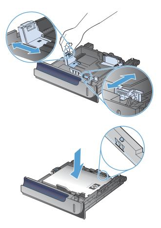
**4.** Slide the tray into the product. The control panel shows the paper type and size.
