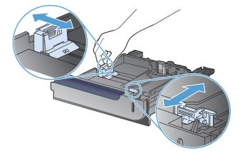
Load paper into the tray face up. Check the paper to verify the guides lightly touch the stack, but do not bend it.
