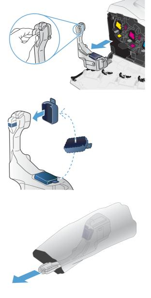
5. Insert the bottom of the new unit into the product first and then push the top of the unit until it clicks into place.
