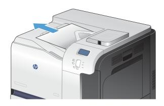
2. If jammed paper is visible in the duplex output area, gently pull it to remove it.
