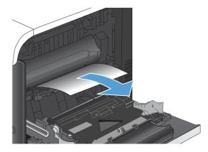
8. If paper is visible entering the bottom of the fuser, gently pull downward to remove it.
