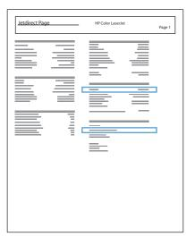
6. **IPv4**: If the IP address is 0.0.0.0, or 192.0.0.192, or 169.254.x.x, you must manually configure the IP address. Otherwise, the network configuration was successful.
