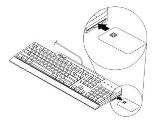
Figure 3. Inserting a smart card into the smart card reader
