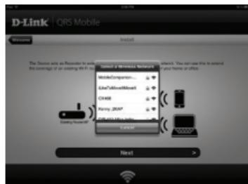
Open QRS Mobile and the Setup Wizard will appear. Tap **Start** to begin. The DAP-1320 will first scan for wireless networks from nearby wireless routers or APs. Select the wireless network that you wish to extend, and enter the password (if required).
