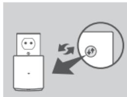
Plug the DAP-1320 into a wall outlet and wait until the power LED is blinking amber. Push the WPS button on the source wireless router or AP, and then push the WPS button on the DAP-1320. The LED will start to flash green.
