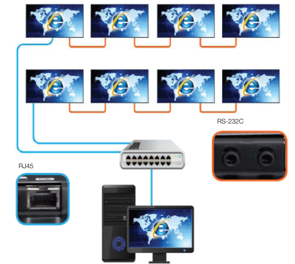
Figure 11. Samsung UDC and UEC LED displays enable RJ45 and RS-232 connectivity simultaneously.
