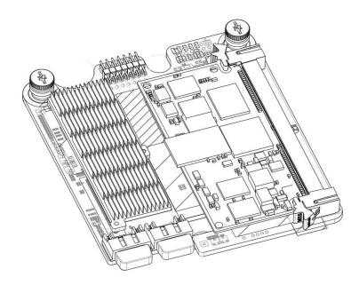
The HP Smart Array P712m mezzanine card is the preferred high value solution for 6Gb/s Shared SAS Storage for the HP ProLiant BladeSystem servers. It is one of the highest performing controllers in the SAS portfolio and provides new levels of reliability for the HP BladeSystem through its support of the latest SCSI technology and advanced RAID capabilities. Supports up to 4 P2000 Smart Arrays.
