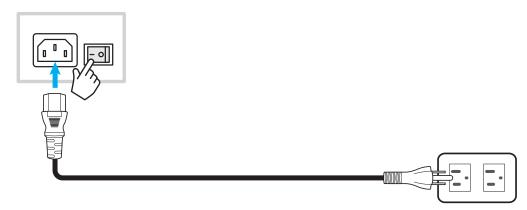
Press the **Power** button to turn on the IFP. The LED indicator light turns white, indicating it is ready to use.
