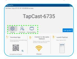
Settings to rename the device, run the **TapCast Pro** app by default after starting the IFP, show or hide the PIN code, and enable or disable split screen (4 screens) feature. Tap **Finish** to save settings and exit the **Settings** menu.
