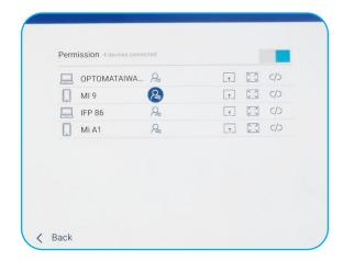
**Grouping Display** to enable or disable the function. If enabled, select devices where you want to share casting screen. Tap **Refresh** to refresh the device list, **OK** to save settings and exit the **Grouping display...** menu, or **Back** to exit without saving.
