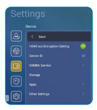
Tap **Device ID** to assign a new ID to the IFP. To confirm, tap **OK**.
