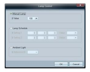
**Lamp Control** is used to adjust the backlight to reduce power consumption.
