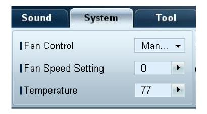
Configure the settings required to detect the fan speed and internal temperature for the product's protection.
