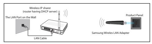
Samsung's Wireless LAN adapter is sold separately and is offered by selected retailers, Ecommerce sites, and Samsungparts.com. Samsung's Wireless LAN adapter supports the IEEE 802.11a/b/g and n communication protocols. Samsung recommends using IEEE 802.11n. When you play video over a network connection, the video may not play smoothly.
