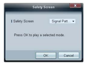
The **Safety Screen** function can be used to prevent screen burn-in when a stationary image displays on the screen of a display device for an extended period of time.
