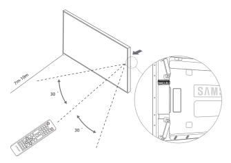
Use the remote control within 7m to 10m from the sensor on the product at an angle of 30° from the left and right.
