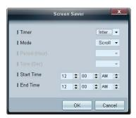
Start Time and End Time can be configured when Interval is selected.
