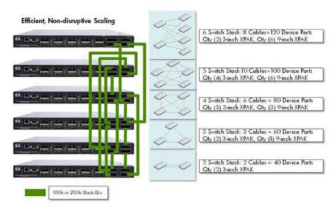
Example of a high availability cable configuration in a single logic FC SAN supporting up
