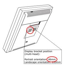
Figure 18: Example of label with position for brackets
