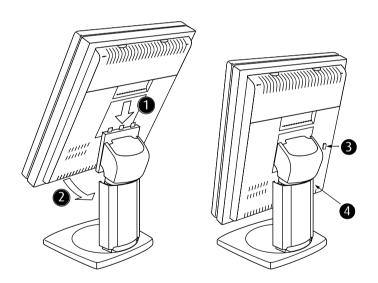
Figure 16: Attaching the panel to the display stand
