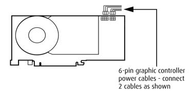
Figure 5: Power connection for the MXRT 7200 controller
