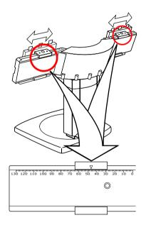
Figure 19: Shift brackets according to label indication
