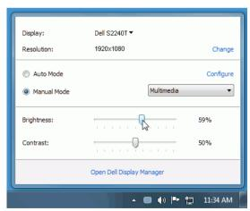
The Quick Settings dialog box also provides access to Dell Display Manager's advanced user interface which is used to adjust Basic functions, configure Auto Mode and access other features.
