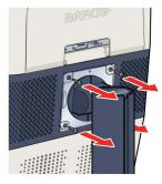
6. Attach the arm stand **firmly** to the panel using 4 screws M4 x 8 mm.
