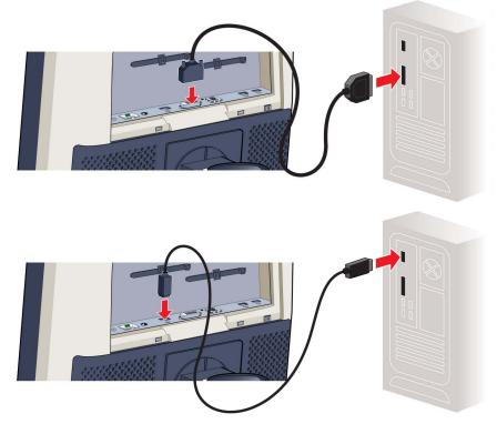
1. Connect the DVI or DP of the display controller to the DVI or DP connector of the display.
