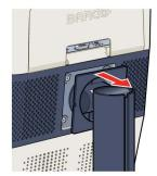
5. Remove the four screws fixing the foot while supporting the foot.
