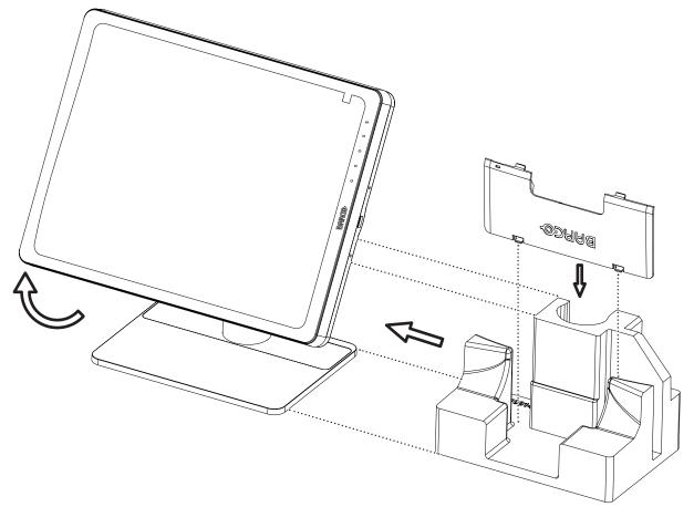
Image 6-2 Placing the protection buffer.
