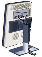
*Tip:* The cable straps at the inside of the connector compartment allow you to fix the cables for better shielding of the cables.
