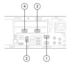
**1 and 2:** Powered Configurable serial port expansion card installation that supplies two additional serial ports (COM3 and COM4) **3 and 4:** Two Power Configurable serial ports, COM1 and COM 2, are standard on the POS System.
