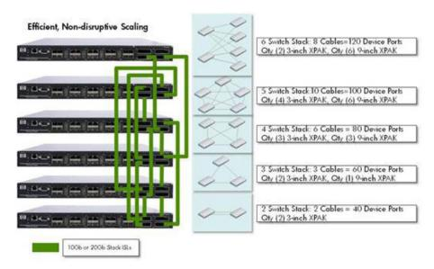
Example of a high availability cable configuration in a single logic FC SAN supporting up
