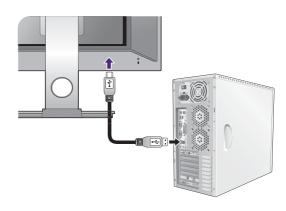
Connect USB devices via other USB ports (downstream) on the monitor. These downstream USB ports transmit data between connected USB devices and the upstream port.
