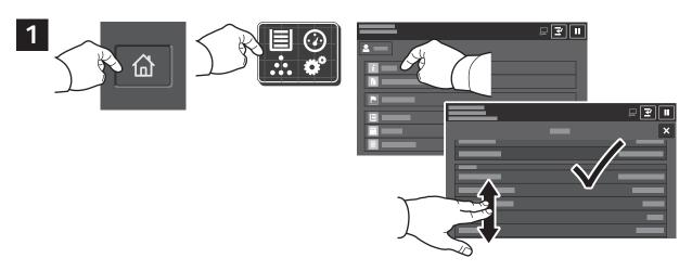
Note the printer IP address on the touch screen. If the IP Address does not appear in the upper left corner of the touch screen, press Home, touch **Device > About** then scroll to check the IP Address.
