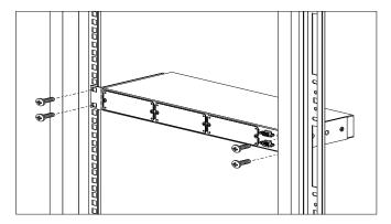
If the Triple Chassis is being installed in a enclosure other than a NetShelter, use the hardware that is appropriate for the enclosure.
