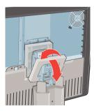
**4** Unscrew the four fixation screws fixing the panel to the stand.
