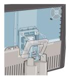
**5** Attach the panel **firmly** to the arm using 4 screws M4 x 10 mm.
