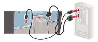
**3** If you want to make use of your display's USB downstream connectors, connect a PC USB downstream connector to the display's USB upstream connector by means of the supplied USB 2.0 cable.
