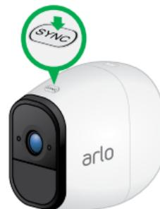
A blue LED on the camera blinks slowly when the sync process starts. A blue LED on the camera blinks rapidly to confirm sync.
