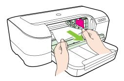
c. Move the carriage to the left, locate any jammed media inside the printer on the right side of the carriage, free any paper scraps or wrinkled media, and pull the media towards you through the top of the printer.
