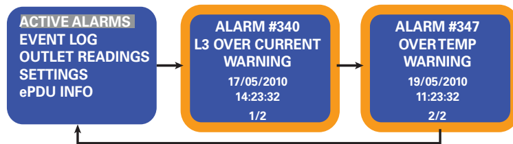
Figure 48. Example Active Alarm Displays
