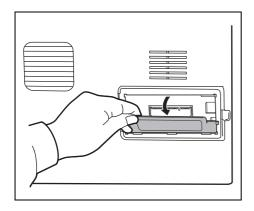
3 Remove the fixing tape in case of the first installation. Then, remove the memory slot cover as shown in the figure.
