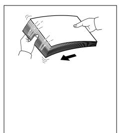
After removing paper from the packaging, fan through the sheets to separate them prior to loading.
