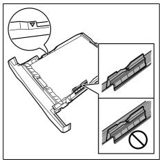
**Note** Do not load paper above the triangle mark located on the width guide.
