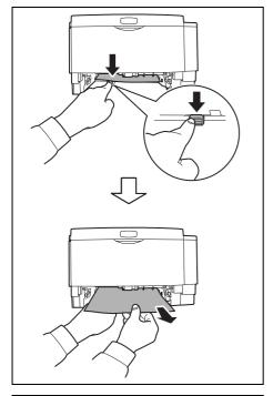
Open the duplexer's cover at the rear of the printer and remove any jammed paper.
