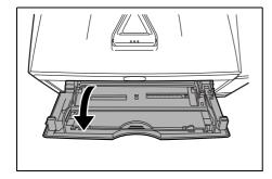
Adjust the position of the paper guides on the MP tray. Standard paper sizes are marked on the MP tray. For standard paper sizes, slide the paper guides to the corresponding mark.
