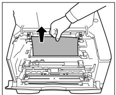
4 If the jammed paper appears to be pinched by rollers, pull it along the normal running direction of the paper.
