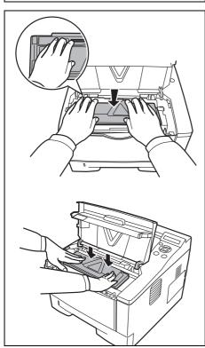
5 Install the new toner container in the printer. Push firmly on the top of the container at the positions marked PUSH, until you hear a click.
