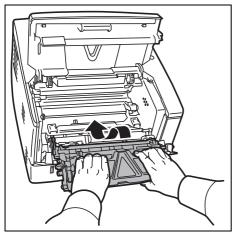
Return the developer unit to its position, aligning the guides at both ends with the slots in the printer. Then, close the front cover and top cover.
