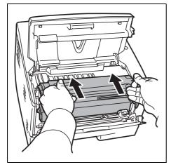
When cleaning is complete, return the drum unit to the original position.
