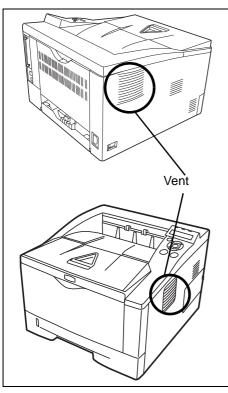
9 Use a lint free cloth to clean dust and dirt away from the vent on the left and the right side of the machine.
