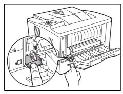
If the paper is jammed inside the fuser unit, open the fuser cover and remove the paper by pulling it out.
