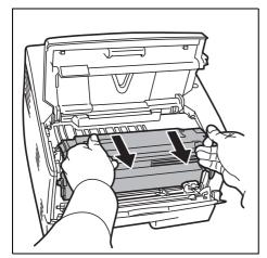
3 Remove the drum unit from the printer by holding the green levers with both hands.
