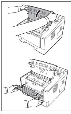
2 Lift the developer unit together with the toner container out of the printer.
