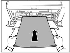
2 Reload the MP tray. Open and close the top cover to clear the error and the printer warms up and resumes printing.
