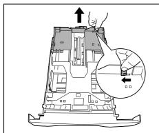
If you are going to use paper that is longer than A4, pull out the extension paper cassette by pushing the release lever one by one and adjust it to the desired paper size.
