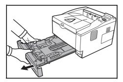
Adjust the position of the width guides located on the left and right sides of the cassette. Press the release button on the left guide and slide the guides to the paper size required, and load the paper into the cassette.
