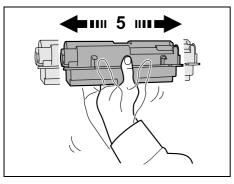
3 Take the new toner container out of the toner kit. Shake the new toner container at least 5 times as shown in the figure in order to distribute the toner evenly inside the container.
