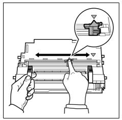
On the drum unit, slide the charger cleaner (green) back and forth 2 or 3 times to clean the charger wire, then return it to its original position (CLEANER HOME POSITION).
