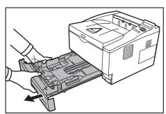
Adjust the position of the width guides located on the left and right sides of the cassette. Press the release button on the left guide and slide the guides to the paper size required.
