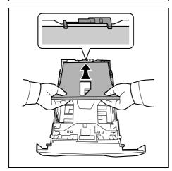
4 Load the paper in the cassette. Ensure the side to be printed is facing down and the paper is not folded, curled, or damaged.
