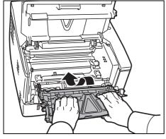
6 Insert the developer unit together with the toner container, back into the machine. Close the top cover and the front cover. The printer warms up and resumes printing.
