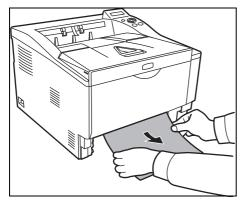
1 Pull the paper cassette all the way out of the printer. Remove any partially fed paper.
