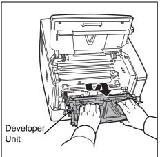
3 Remove the drum unit from the printer by holding the green levers with both hands.
