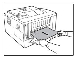
1 Open the rear cover and remove the jammed paper by pulling it out.
