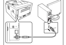
Connect the other end of the USB cable to the computer's USB interface connector.
