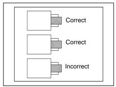
When loading envelope, place with the envelope flap closed and keep the printing side face-up. Insert envelope against the guide with the flap on the front or left side until they stop.
