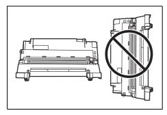
4 Place the drum unit flat on a clean, level surface.
