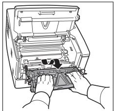
2 Open the top cover and front cover, and lift the developer unit together with the toner container out of the printer.
