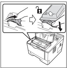
2 Turn the lock lever to the unlock position. Push the lock lever to the position marked by the arrow and pull out the toner container.
