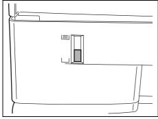
There is a paper gauge on the left side of the front of the paper cassette to indicate the remaining paper supply. When paper is exhausted, the pointer will go down to the level of (empty).
