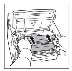
5 Return the drum unit to its position, aligning the guides at both ends with the slots in the printer.
