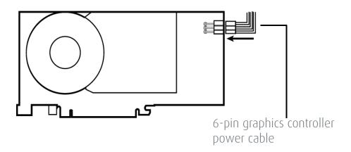
Power connection for the MXRT 7300 & MXRT 7400 controllers
