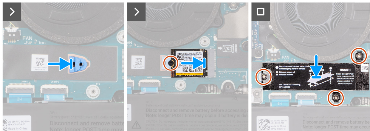
Figure 28. Installing the M.2 2230 SSD
