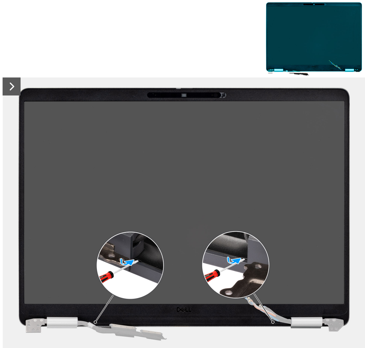
Figure 61. Prying the plastic bezel
