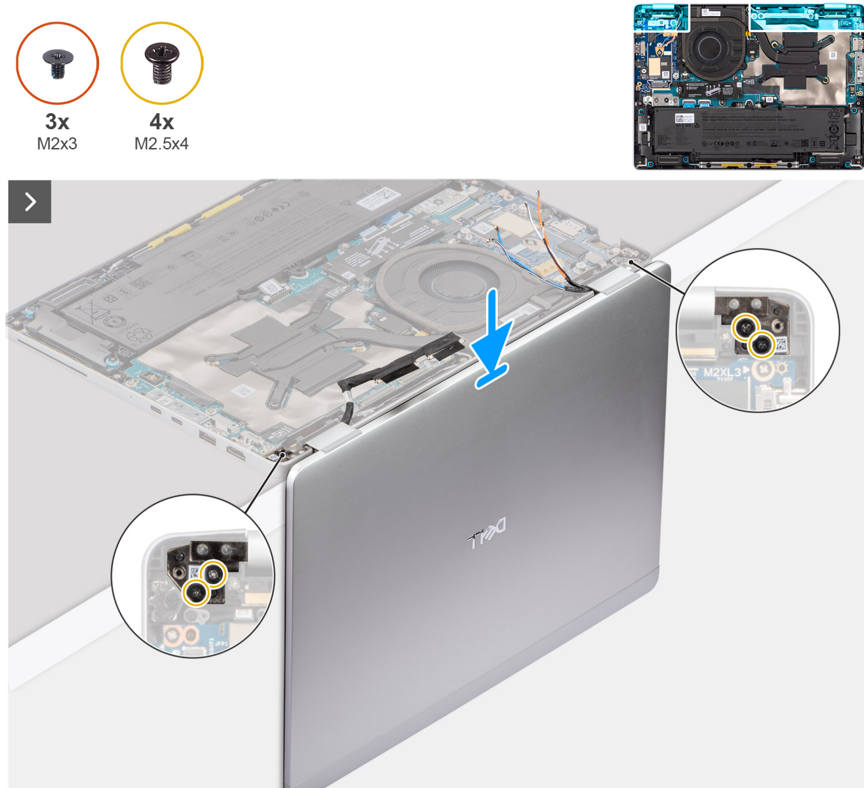
Figure 59. Aligning the display assembly with the palm-rest assembly
