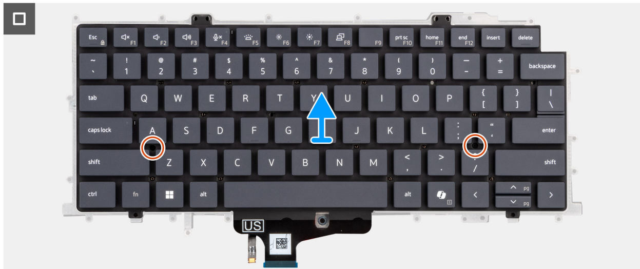
Figure 94. Removing the keyboard
