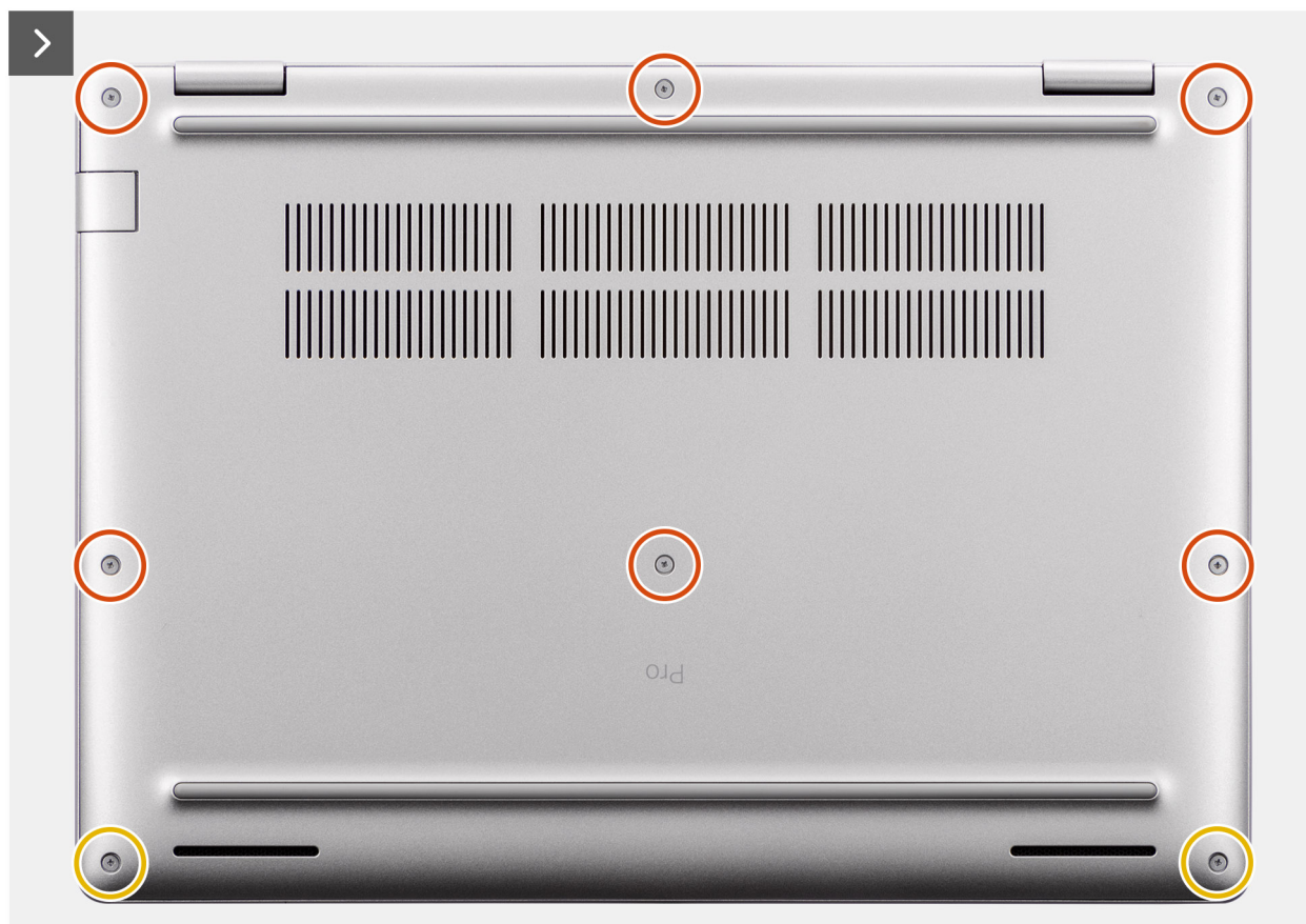
Figure 17. Removing the base cover
