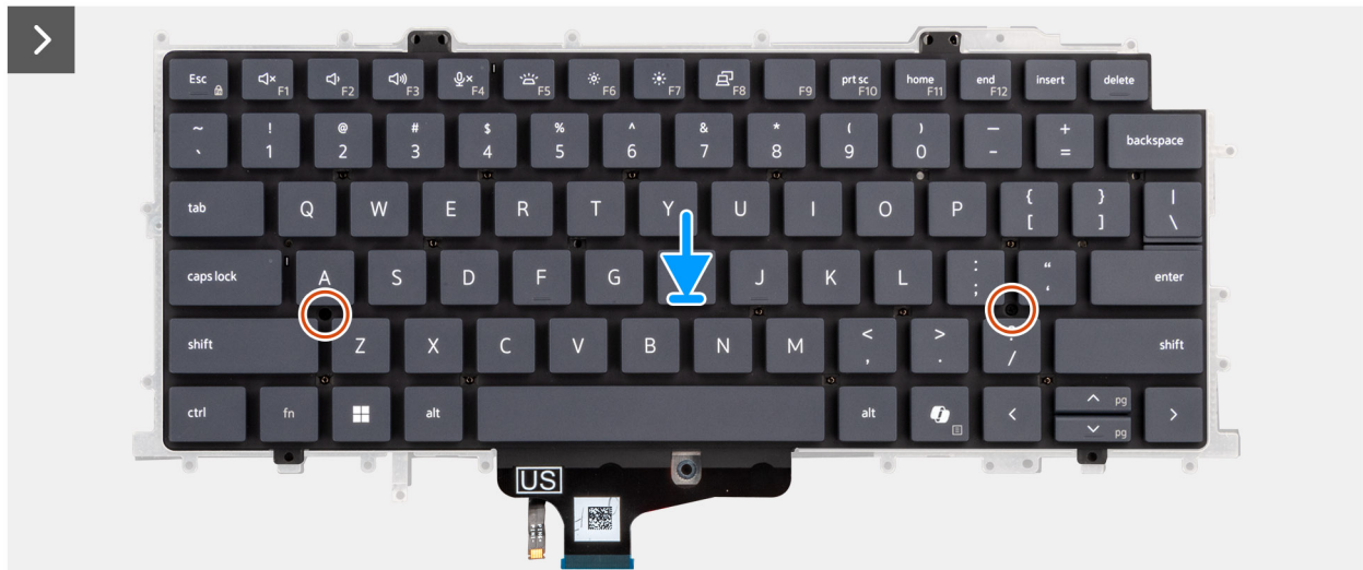
Figure 95. Installing the keyboard
