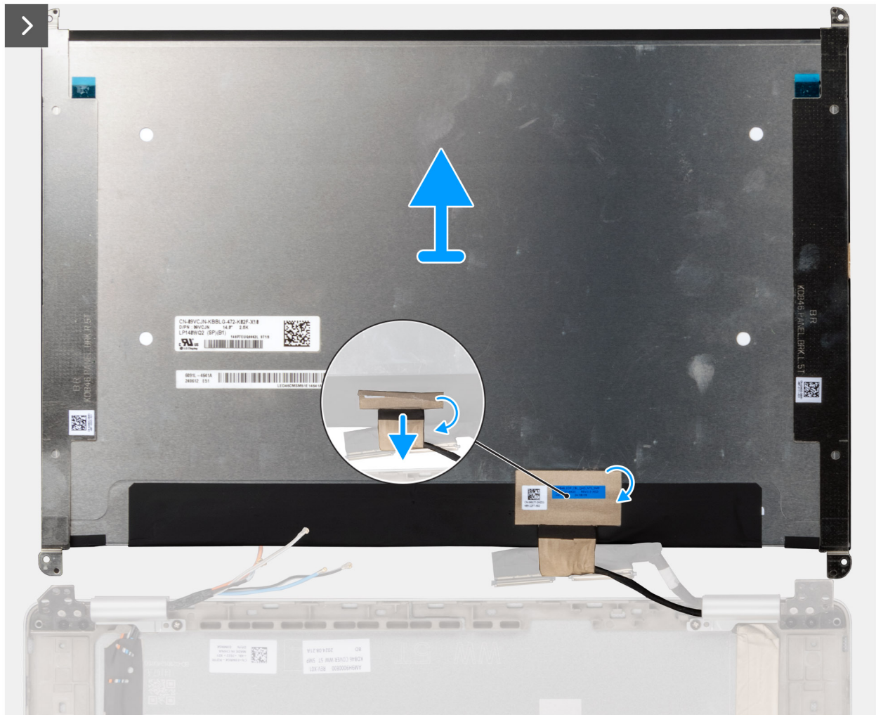
Figure 69. Removing the display panel
