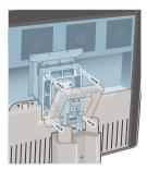
**5** Attach the panel **firmly** to the arm using 4 screws M4 x 10 mm.
