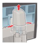
**3** Lift the plastic frame that covers the fixation of the panel to the stand. Turn it for 45 degrees to uncover the fixation screws.
