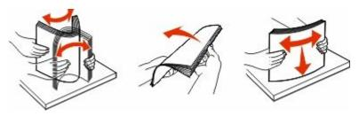
**4** Load the paper stack with the recommended print side faceup. Load the paper in either the long-edge or short-edge orientation as shown.
