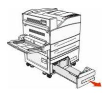
**2** Squeeze the length guide tab inward as shown, and slide the guide to the correct position for the paper size being loaded.
