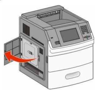
**2** Loosen the screw(s) on the system board cover.
