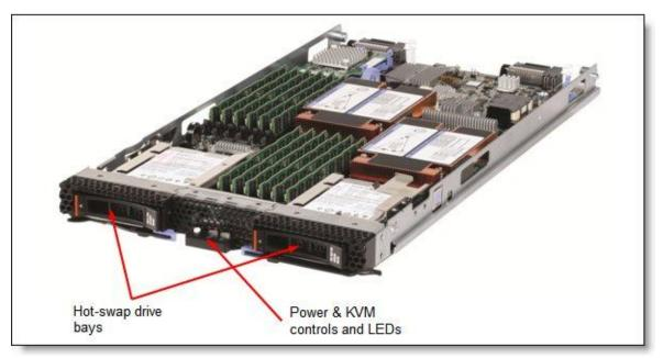
Figure 2. Front view of the IBM BladeCenter HS23E
