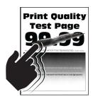
**Note:** Before solving the problem, print the Print Quality Test Pages. From the control panel, navigate to **Settings** > **Troubleshooting** > **Print Quality Test Pages**. For non-touch-screen printer models, press **OK** to navigate through the settings.
