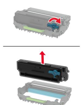
**4** Unpack the new imaging unit, and then insert the toner cartridge until it *clicks* into place.
