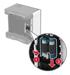
**9** Apply isopropyl alcohol to a soft, lint-free cloth, and then wipe the pick roller assembly.
