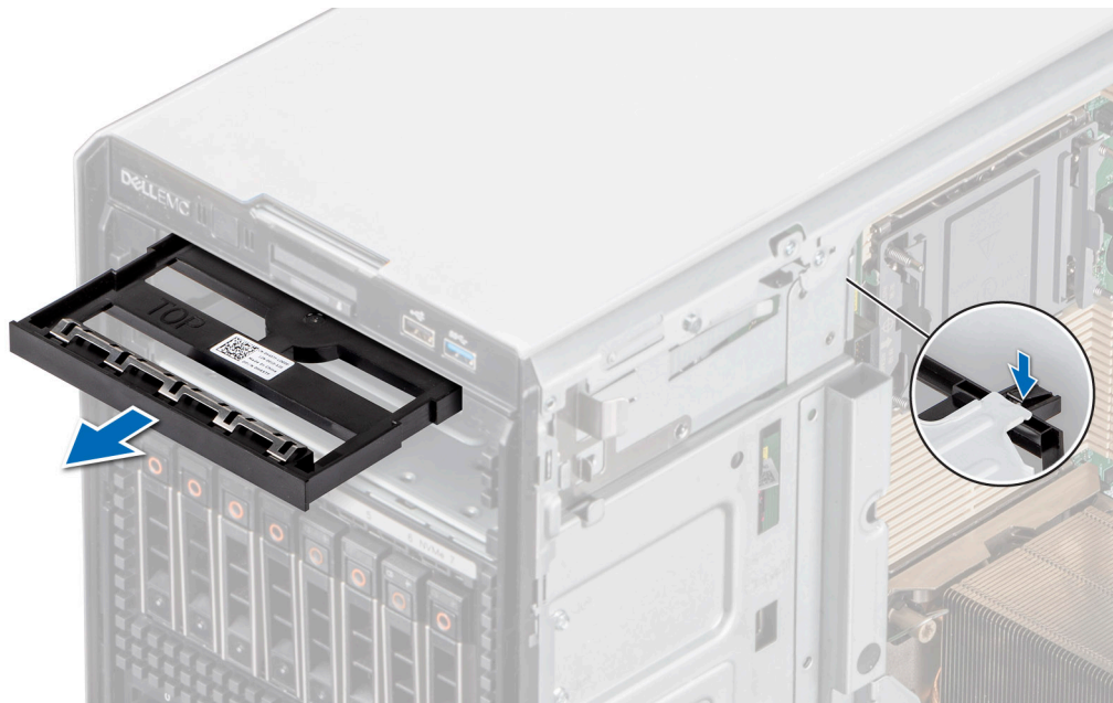
Figure 93. Removing the optical drive blank
