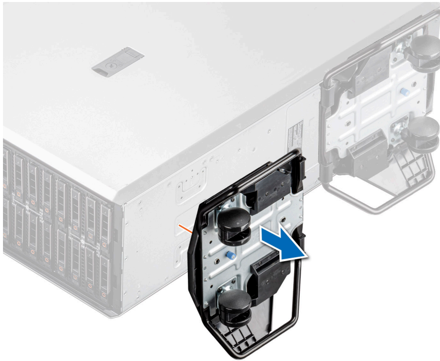
Figure 29. Removing caster wheels
