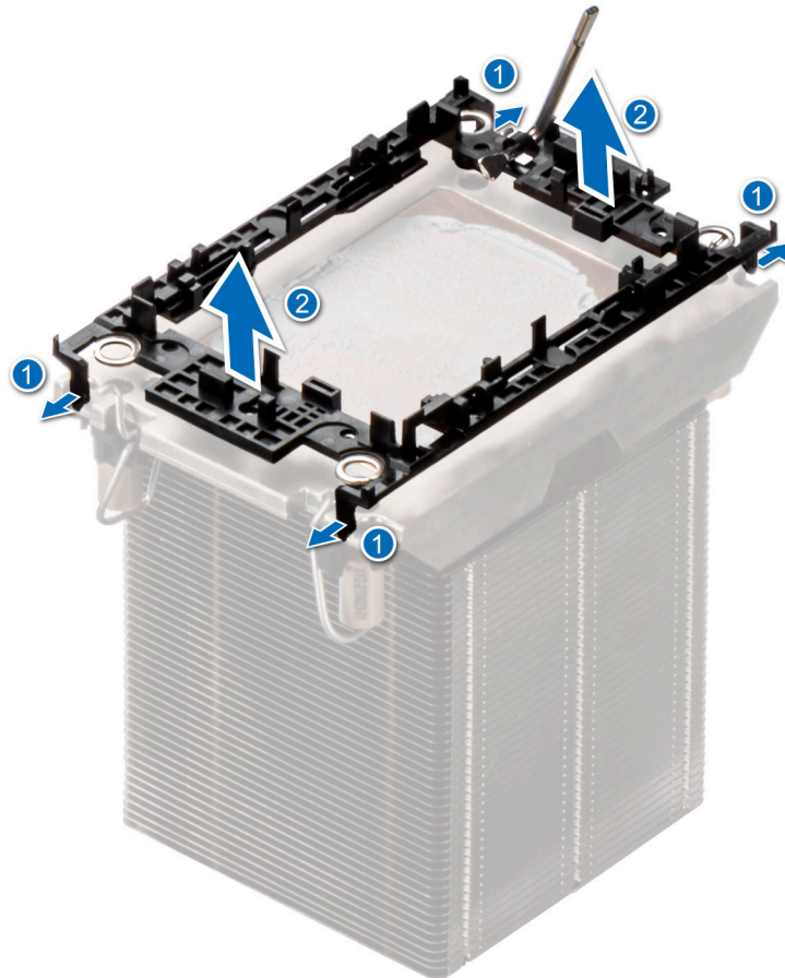
Figure 143. Removing the retaining clip
