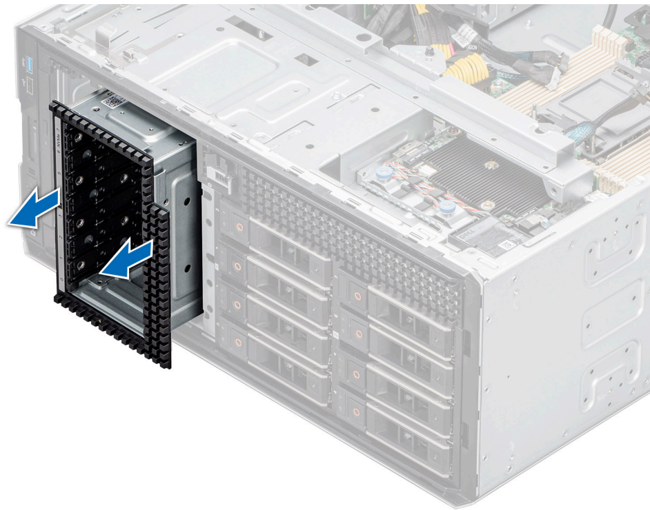
Figure 68. Removing a NVMe drive bay
