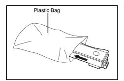
**3** Put the old toner container in the plastic bag (contained in the toner kit) and discard it later according to the local code or regulations for waste disposal.
