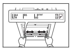
4 Adjust the position of the paper guides on the MP tray. Standard paper sizes are marked on the MP tray. For standard paper sizes, slide the guides to the position marked correspondingly.
