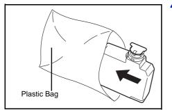
**4** To prevent toner from spilling, put the old waste toner box in the plastic bag (contained in the toner kit) and discard it later according to the local code or regulations for waste disposal.
