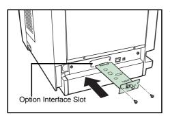
The network interface kit is a high-speed interface for communications speeds of 1 gigabit per second. In addition to the TCP/IP and NetBEUI supported by the machine's standard network interface, it also supports IPX/SPX and Apple Talk, so network printing becomes possible in various environments, including Windows, Macintosh, UNIX and Netware. For details, refer to *IB-50 User's Manual*.
