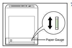
7 Insert the paper cassette into the slot in the printer. Push it straight in as far as it will go.
