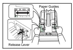
4 Pull the release lever of both side guides and slide to the desired paper size.
