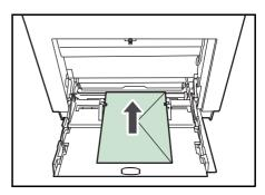
Normally, envelopes have a diagonal grain direction. Refer to *Paper Grain on page 2-6*. This direction can easily cause wrinkles and creases when envelopes pass through the printer. Before purchasing envelopes, make a test print to check whether the printer accepts the envelope.
