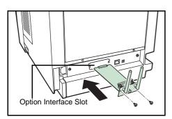
This is a wireless network interface kit which supports the wireless network specifications IEEE802.11n (Max 300 Mbps) and 11 g/b.
