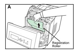
**3** If the paper has jammed near the registration roller, as shown in **A**, remove the paper by pulling it up from the center.
