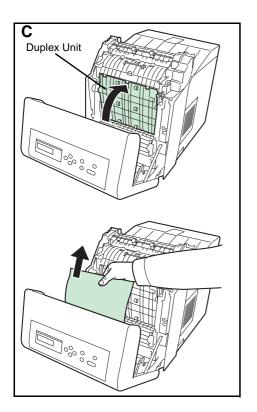
If the paper has jammed inside the duplex unit, as shown in **C**, lift the duplex unit and remove the paper by holding it in the middle.
