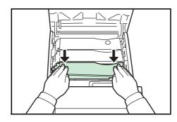
7 Push down on the top of the toner container to install it firmly in place. Use the same procedure to replace the other color toner containers.
