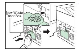
6 Insert the new waste toner box as shown in the figure. When the box is set correctly, it will snap into place.
