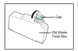
3 Close the cap to the old waste toner box after removing the box from the printer.
