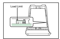
**Note** Do not load more paper than will fit under the load limits on the paper guides.
