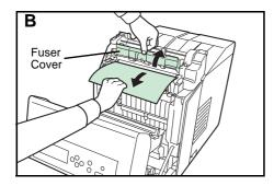
If the paper has jammed inside the fuser unit, as shown in **B**, open the fuser cover and remove the paper by pulling its edge.
