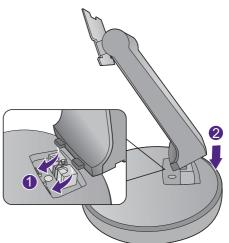
Tighten the thumbscrew on the bottom of the monitor base as illustrated.
