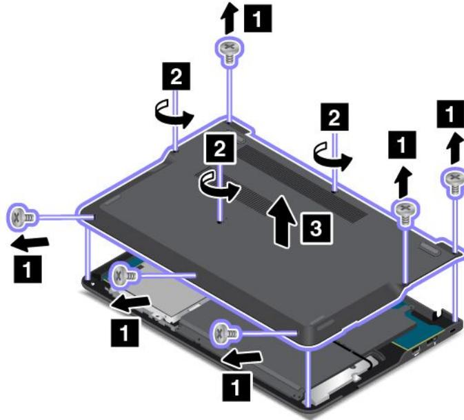
4. Install the new base cover assembly **1**, then tighten the three screws **2**, and then install the six screws **3**.
