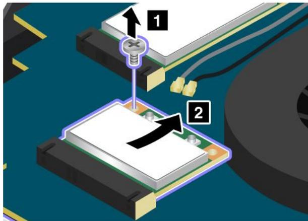
6. Align the contact edge of the new card with the corresponding socket **1**. Pivot the card until you can snap it into place. Secure the card with the screw **2**.
