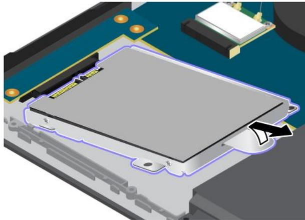
6. Place the new hard disk drive or solid-state drive into the drive bay.
