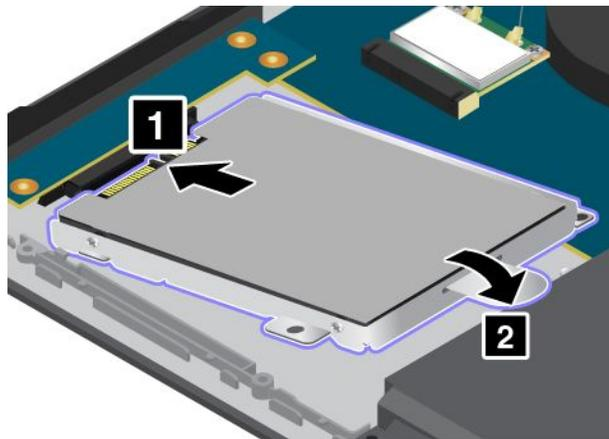
7. Slide the hard disk drive or solid-state drive horizontally and firmly into the connector **1**. Ensure that the hard disk drive or solid-state drive is correctly seated in the bay and secured by the hook **a**. Then reinstall the screws **2**.
