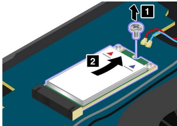
6. Align the contact edge of the new WAN card with the corresponding socket **1**. Pivot the WAN card until you can snap it into place. Secure the WAN card with the screw **2**.
