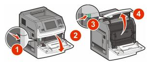
2 Lift and pull the print cartridge out of the printer.
