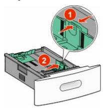
2 Unlock the length guide, squeeze the length guide tab inward, and slide it to fit the paper size being loaded.
